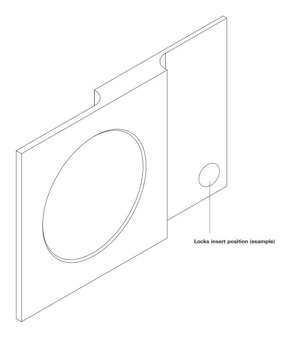
NOTES: Handles are sent as is, own metalworks are needed to insert desired locks
