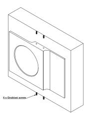
Push MDV plate against door surface and tighten the 4 grub/set screws (using supplied Allen/Hex key) to fix MDV plate in place
