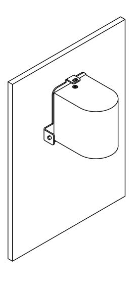
Step 4 - Install elbow shade onto wall bracket
