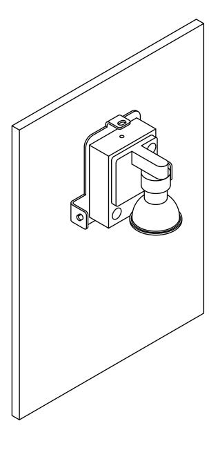
Step 3 - Install lamp housing onto lamp frame
