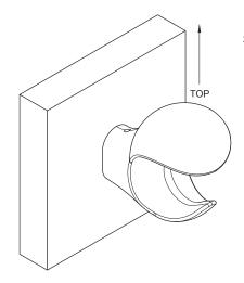
2. Thread ball hook onto the M4 thread of the hanger bolt using the top hole of the ball hook. When the ball hook touches the wall ensure that the ball hook is aligned vertically and the back face of the hook is flush to the wall.
